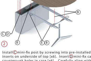
inserts on underside of top [x6]. Insert mini-fix cams in countersunk holes in case [x6]. Carefully align with case and set top in place- turn mini-fix cam to lock into position. Using B1/4"-20 x 7/8" joiner bolts [x15] fasten rail brackets, case bracket and leg to top.
