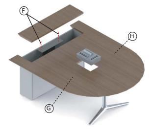
Align threaded inserts in lid with through holes in top plate of lift. Secure with (F) 1/4"-20 x 3" socket head cap screws. Note, the lid is meant to be loose- this is to ensure fingers are not pinched during operation-see lift guide for further safety details.
