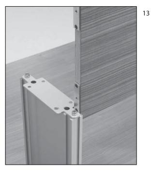
Wood gallery panels: Slide the t-nuts into the groove on the extrusion. The panel needs to be placed in the extrusion closest to the approach side of the desk.
