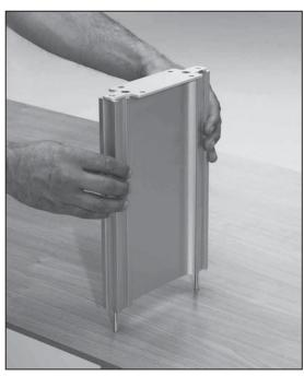
· Slide the gallery post assembly over the treaded rods. The threaded rods need to pass through the holes in the bracket but only enough for the lock nut to fasten. If the rod is to tall the gallery top won't seat correctly. Adjust the threaded rods appropriately.
