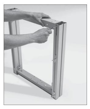
• Screw one mini-fix connecting rod into the hole on each t-slot nut (located at the top, middle & bottom of the base).
