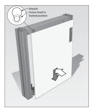
Place the head of the screws thru the keyslot found on the base bracket. Allow the panel to drop down and seat itself in the keyslot.
