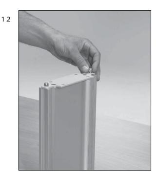
Place the 1/4"-20 lock nuts on to the ends of the treaded rods and hand tighten. In some cases you may need to loosen the nuts on the post to allow the panel to slide in easier.
